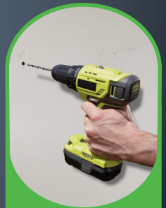
Simply drill 1/4 in. hole and push cable through wall or microduct.
