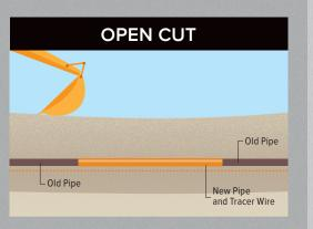
expose existing or install new utilities where there are no buildings or other obstructions, then backfilling the trench.
