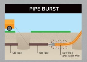
Pipe bursting is a trenchless method of replacing old buried pipes with new replacement pipe by bursting the old pipe and pulling new pipe in its place.
