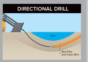
Directional drilling is a trenchless method of installing underground utilities that involves drilling along a chosen bore path to install utilities that need to go under roads, sidewalks, or other obstructions.
