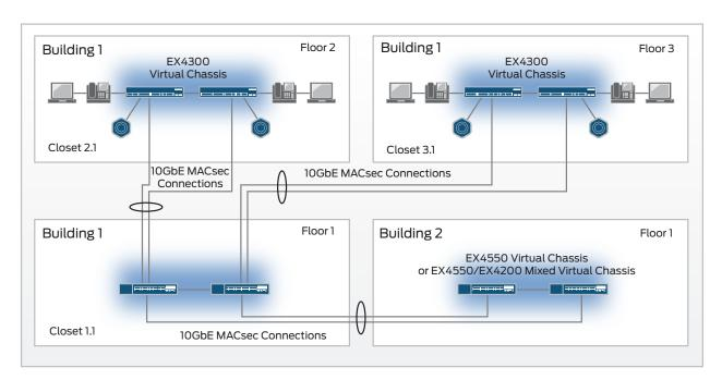
Figure 7: MACsec deployment with EX4300 and EX4550 switches.
