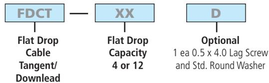
**Ordering Example:** To hold up to 12 flat drop cables, with lag screw hardware kit included, order part number FDCT-12D.
