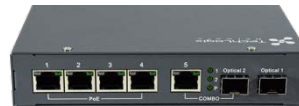
TL-NS42-POE Four port unmanaged switch with 30W PoE per channel. Includes one twisted pair and two SFP uplink ports for daisy-chaining over fiber.
