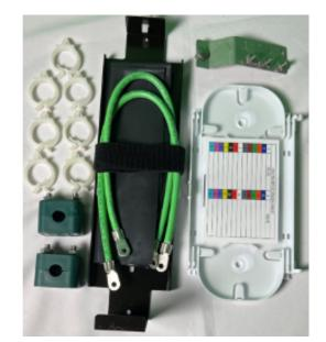
Add-on kit for expressing and splicing most 8" or wider pedestals. The kit includes 24 fiber splice tray, splice tray mounting kit for up to six 1/2" thick splice trays, 1 ground bar, 2 ground straps, # 6 ground wire clamp, cable clamps, tie off bracket, and wire saddles.
