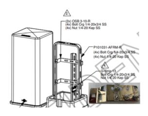
10" HDPE solid base pedestal with 2 OSB 3-10R Brackets for mounting adapter plates, splice tray bracket, cable clamps, and securing drop cables.
