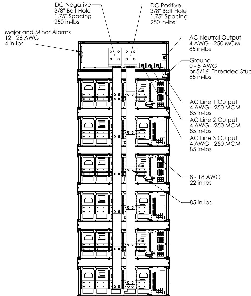
\*\*Phase 3 connections not applicable for bi-phase inverters
